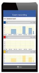
When a value greater than the threshold is measured, the time of occurrence, end time, and the maximum value for that period are recorded.
