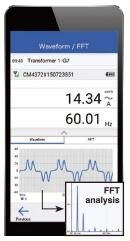
Waveforms such as current and voltage, and FFT analysis waveforms can be displayed.
