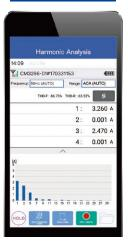
Calculate and display harmonic levels for individual orders, content percentages, and total harmonic distortion (THD-F and THDR). Waveform observation/ FFT analysis
