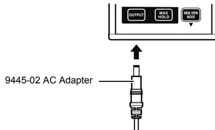
2. Connect the AC adapter plug to an AC wall outlet.
