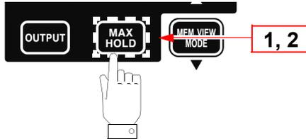
1. Press **MAX HOLD** to hold the maximum value of the resultant RMS value R and the **MAX** icon lights.
