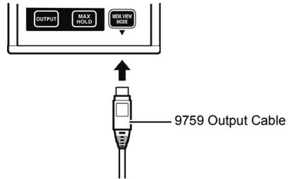
2. Connect the output cable plug in the oscilloscope, recorder, or etc. connector.
