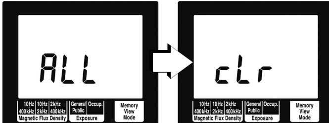
After this it displays the model number and estimated remaining battery life, and is restarted using the factory default settings.
