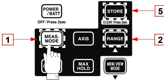
1. Press **MEAS. MODE** to open the exposure level (Occup.) mode screen. Occup. Exposure is selected.
