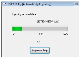
The data recorded in the logger is imported to the computer automatically. Imported data is saved to a file (Auto Import).
