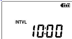
4 Select the recording interval for the logger (in this case, 10 minutes).
