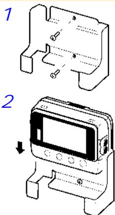
1 Mount the LR9901 to the wall using the two screws.
