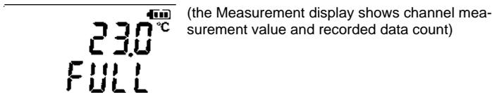
When memory becomes full during endless recording, the recorded data count (equal to the memory capacity) remains constant.
