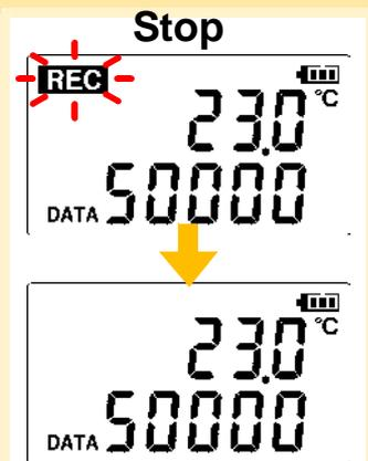
**Start** From the Measurement display, hold the **REC/STOP** button for two seconds.
