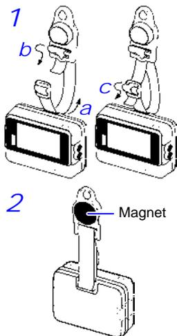
1 Attach the Z5004 to the strap/stand attachment hole.
